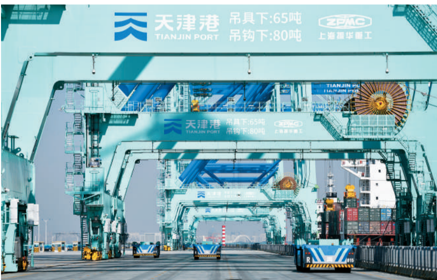
Artificial Intelligence Robot of Transportation (ART) at the smart and zero carbon container terminal at Section C of Beijing Port Area of Tianjin Port. (PHOTO: XINHUA)
